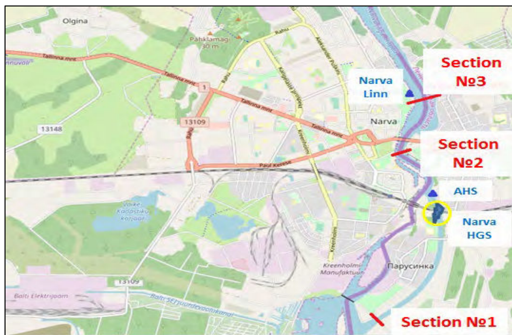
Figure 4.2.3 Hydrometric gauging sections on the Narva River below the Narva HGS.
