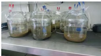
Figure 4.3.4 Sediment biotest with amphipods. Test organisms: Monoporeia affinis , Pontogammarus robustoides .
